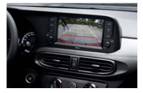
A rear camera watches your back and conveys the image to the 8-in touchscreen (GLS standard equipment). A graphic overlay on the screen acts as a parking assistant helping the driver avoid curb rash on the wheel rims and bumper scratches.
